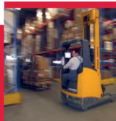
An integrated forklift control system with modern radio terminals reduces distances and optimizes workflows.
